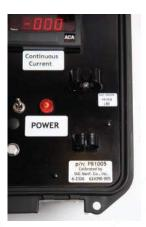
Determine the allowed voltage based on the cable length using the chart provided inside the lid of the unit. See page 4 for details.
