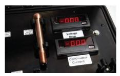
Voltage Drop readings equal to or less than for the cable specs on the chart indicate that the ground cable assembly is good.
