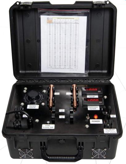
Make sure the Current Control dial is turned fully counterclockwise to zero.
